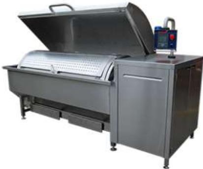
The filled bags are loaded directly into the product chiller, where they gently tumble in circulating cold water. The tumbling action quickly removes heat from the bags, dropping the product temperature from 82°C to 5°C in 60 minutes or less.
